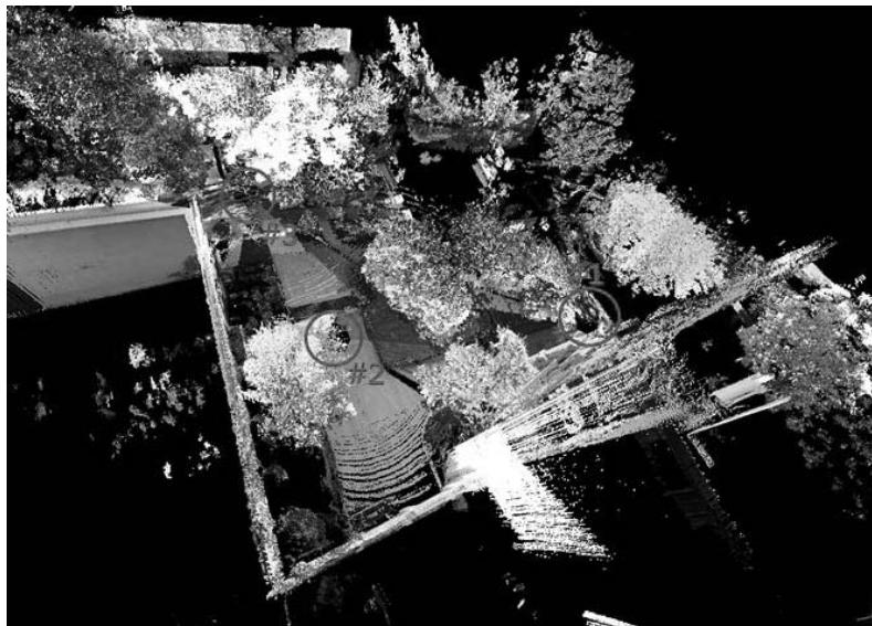
Fig. 9: Registered point cloud
